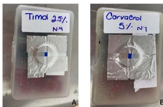
Figure 2. Boxes containing blackberries and raspberries adapted for headspace sampling. (A) PLA/ \beta -CD-thymol, 2.5% wt%; (B) PLA/ \beta -CD-carvacrol, 5.0%.
